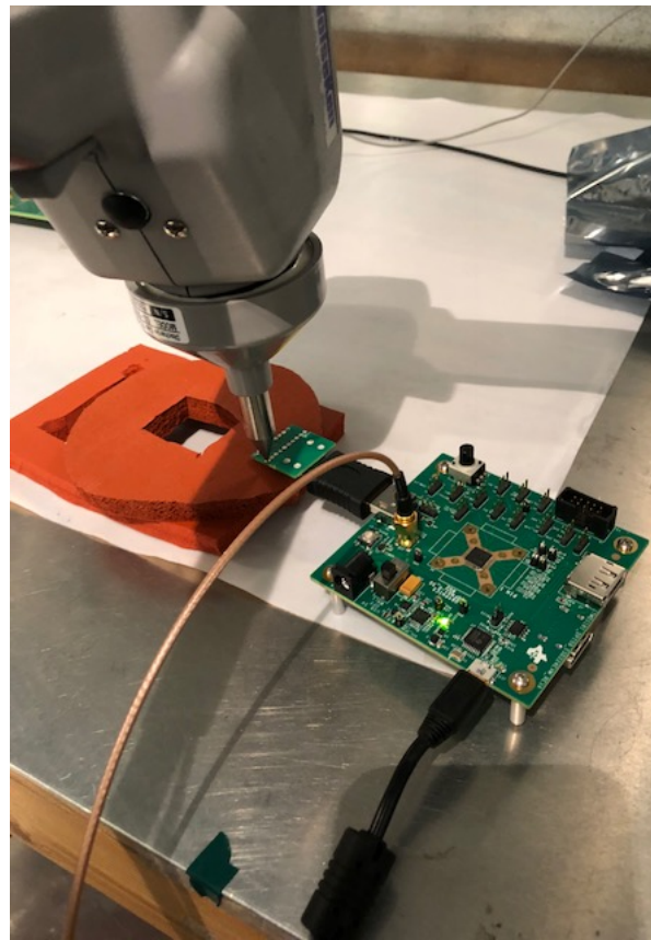
Figure 16. ESD Test Setup
