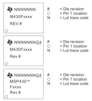
NOTE: Package marking with "TM" applies only to devices released after 2011.
