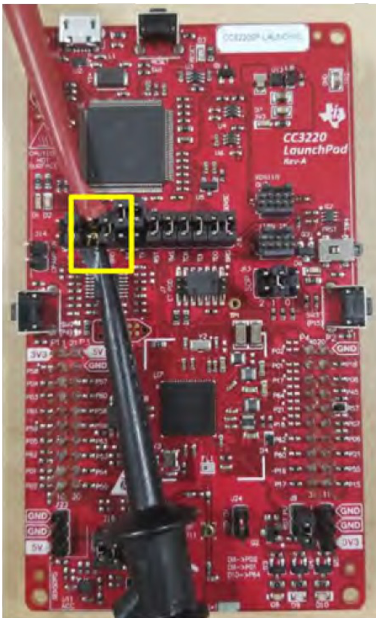
Figure 3-25. Probe Connection for Power Measurement
