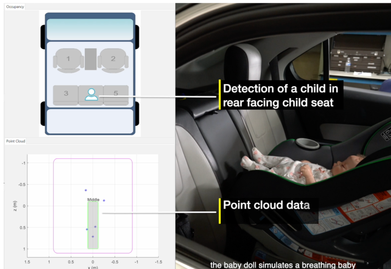
Figure 5. Detection of a child (a baby doll simulating a breathing child) in the rear seat of a vehicle ( video )
