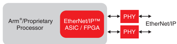
Figure 8. Integrated EtherNet/IP with processor.
