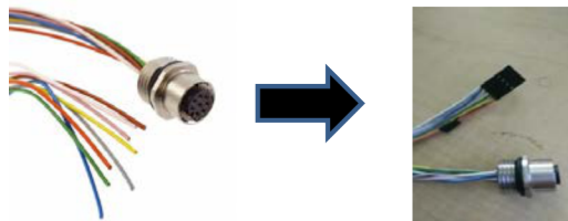
Figure 9. Adapter to Connect the Heidenhain Cable to IDDK
