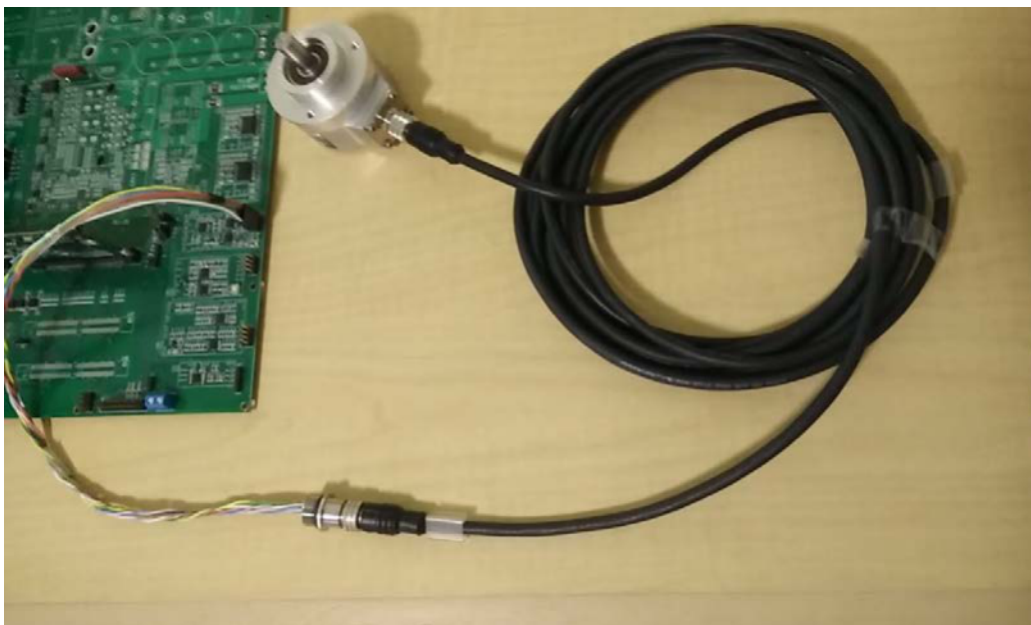
Figure 10. M12 Heidenhain Cable Connects to the Encoder
