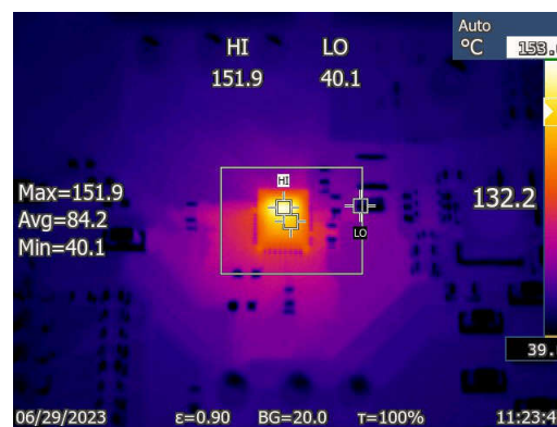
Figure 3-4. Thermal Image of DRV8317 at 50kHz PWM Frequency and 2.99A RMS
