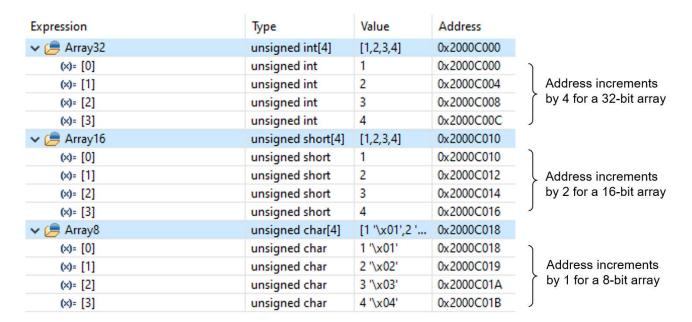
Figure 3-2. Memory Allocation in Arm Core
