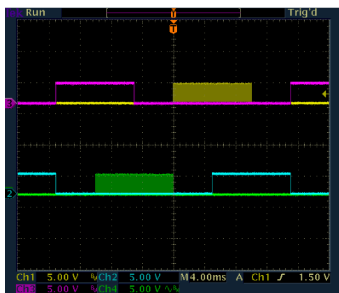
Figure 12. The PWM Outputs: PWM 1 (Yellow), PWM 2 (Pink) and PWM 5 (Green), PWM 6 (Blue)
