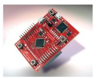
microcontroller's USB 2.0 Device interface, Hibernation module, Motion Control PWMs and overall cost effectiveness.
