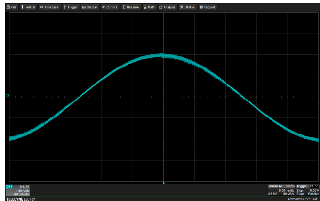
Figure 23. Current Waveform With 1/256 Microstepping, Smart Tune Ripple Control
