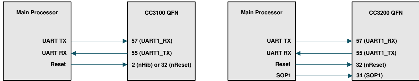
Figure 3-1. CC3200 and CC3200 QFN Programming Setup
