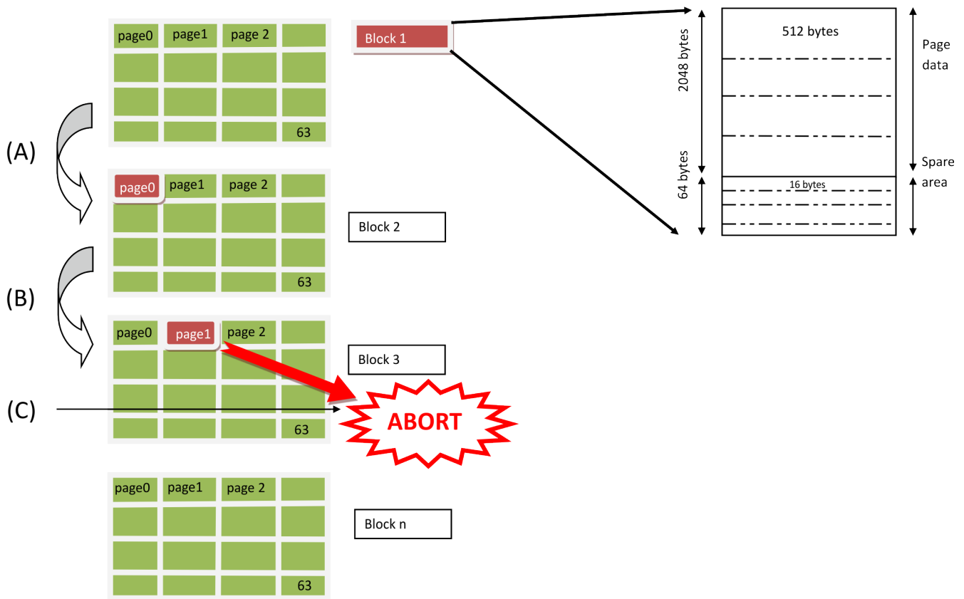
Figure 11. D800K008 ROM Behavior Before Application of Software Patch (1)
